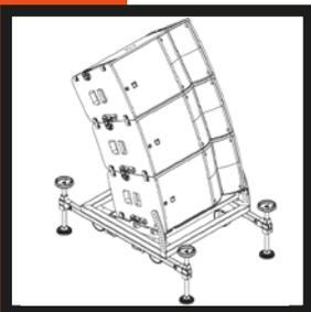
dolly can also be used as a groundstackframe with adjustable angle and even K2-JACK is compatible for maximum stability
